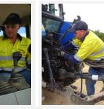
When connecting / disconnecting hydraulic lines ensure you have released the oil first.
